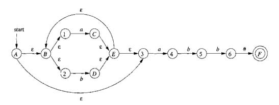
Figure 3.57: NFA constructed by Algorithm 3.23 for (a|b)\*abb#
