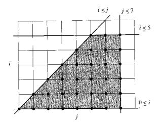
Figure 11.11: The iteration space of Example 11.6
