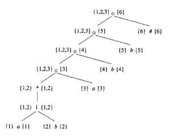
Figure 3.59: firstpos and lastpos for nodes in the syntax tree for  $(\mathbf{a}|\mathbf{b})^*\mathbf{abb}\#$
