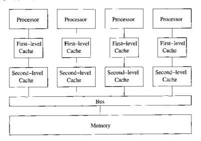
Figure 11.1: The symmetric multi-processor architecture
