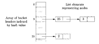
Figure 6.7: Data structure for scarching buckets
