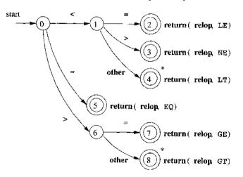
Figure 3.13: Transition diagram for relop
