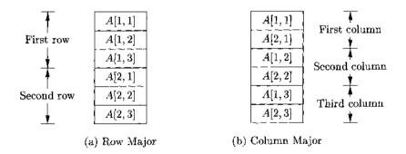
Figure 6.21: Layouts for a two-dimensional array.
