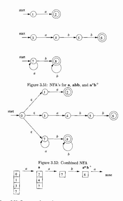
Figure 3.53: Sequence of sets of states entered when processing input aaba
