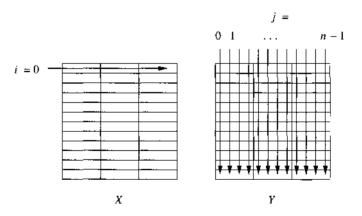
Figure 11.6: The data access pattern in matrix multiply
