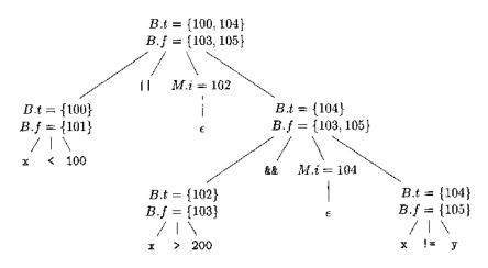
Figure 6.44: Annotated parse tree for  $x < 100 \parallel x > 200 \&\& x ! = y$
