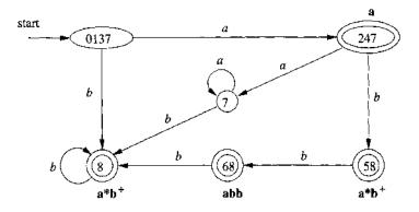
Figure 3.54: Transition graph for DFA handling the patterns  $\mathbf{a}$ ,  $\mathbf{abb}$ , and  $\mathbf{a^*b^+}$
