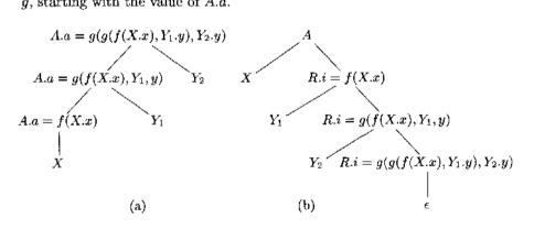
Figure 5.23: Eliminating left recursion from a postfix SDT
