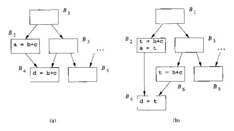
Figure 9.31:  $B_3 \rightarrow B_4$  is a critical edge
