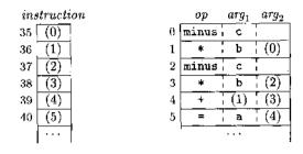
Figure 6.12: Indirect triples representation of three-address code
