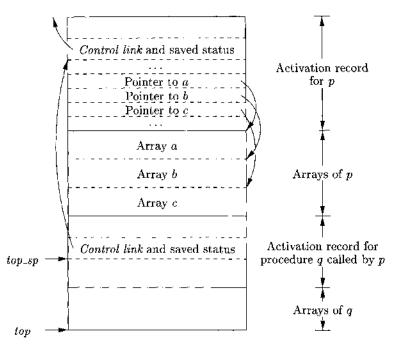
Figure 7.8: Access to dynamically allocated arrays
