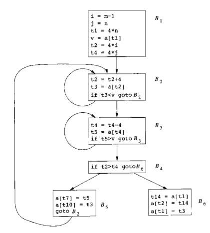
Figure 9.9: Flow graph after induction-variable elimination
